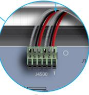
J4500 Detail: Fig. 2.3 shows the connections for a single-lane drive-thru.
