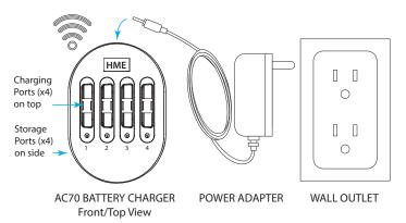
**Note**: Only use the HME approved Power Adapter provided Storage ports do not charge batteries.
