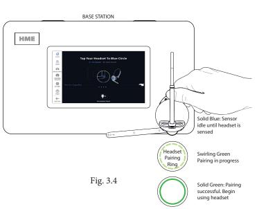
Note: If pairing fails (indicated by a red swirling ring), try again. Hold the headset steadily centered and flush against the Headset Pairing Ring (headset movement and distance from the Pairing Ring can cause pairing errors).
